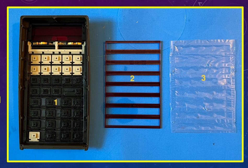
Exquisite manufacture, with the double injected keys, where other manufacturers used painted keys.
